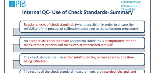
The limits are used to establish process uncertainties and to control future measurement performance.
